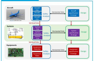
Exchanges between design and safety activities (ARP4754A) exist at aircraft, system and equipment level. Current activities are focused on System level, and preliminary development phase.
